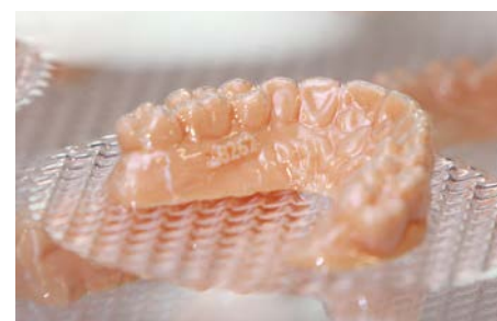
NimroDENTAL can now 3D print ortho-study models much faster than they could make traditional plaster models.
